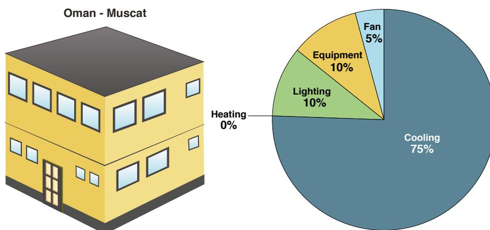
**Figure 3.** (a) 3-D rendering for energy model, (b) annual energy end-use distribution for a prototypical villa in Muscat.
