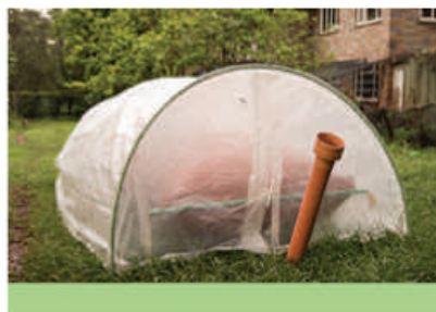
Tubular biogas system
