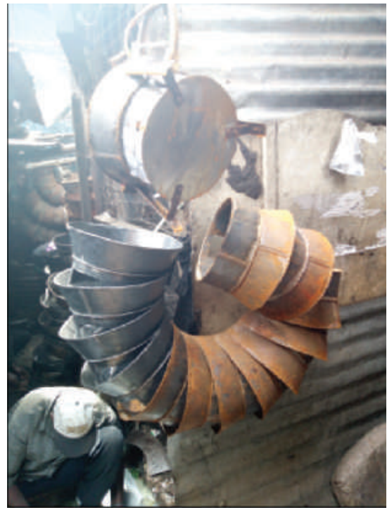
Figure 28: A Jua Kali artisan working on parts the KCJ metal cladding at Kamukunji
