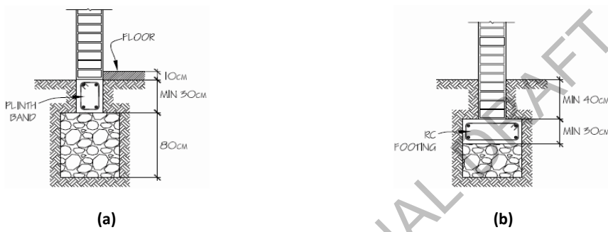
Figure 6.7.17 Foundation construction: (a) RC plinth band and stone masonry foundation; (b) RC strip footing
