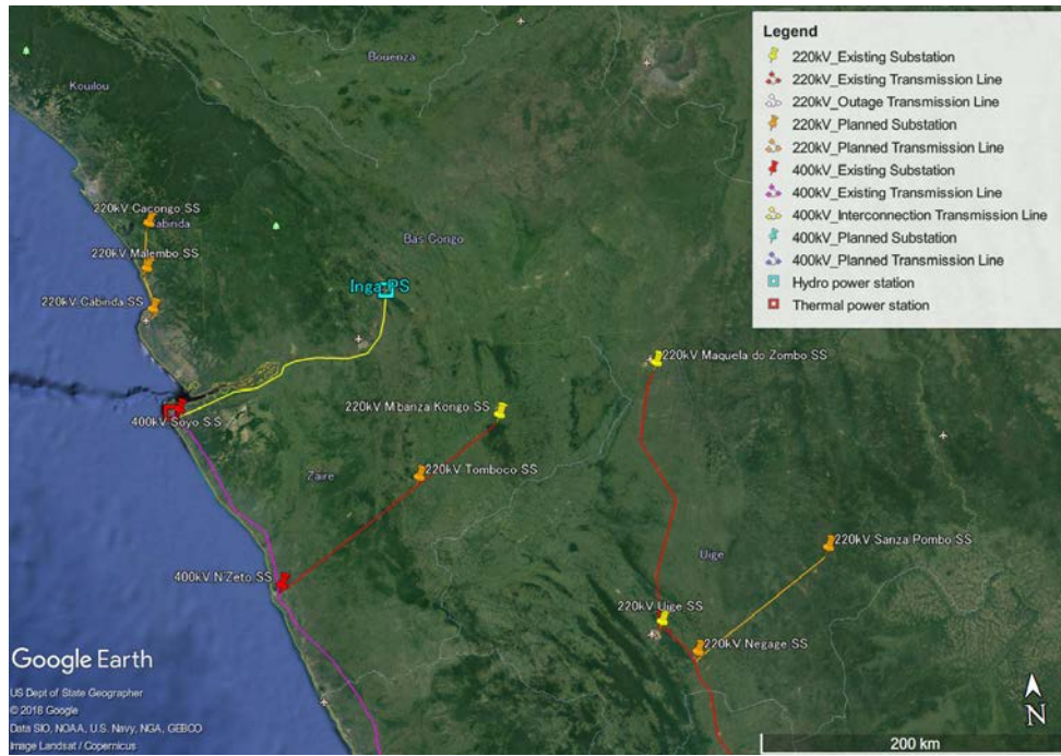
Figure 7-28 System connection status of Soyo thermal power station
